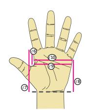
**Length** ( $\ell$ )6 - Length from the base of the index finger to the thumb webbing with the thumb in a relaxed postion.
