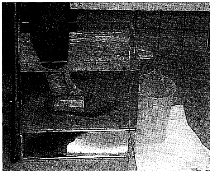
FIGURE 1: Standardized water displacement technique.
